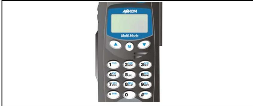
**Figure 6: System Radio Front Panel**
