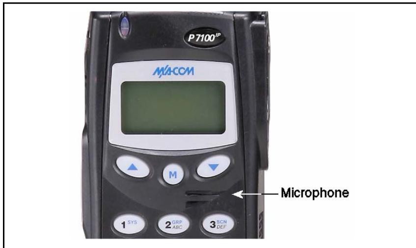
Figure 21: Radio Microphone
